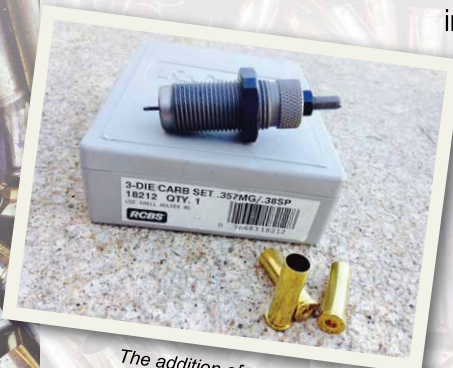
The addition of a carbide steel insert, into the bottom of the resizing die, made reloading both the 38 Special and 357 Magnum a lot easier.
