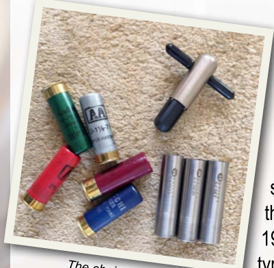
The choice of choke and shells (shot size, hardness, velocity and weight of shot charge) is keenly important to success.
