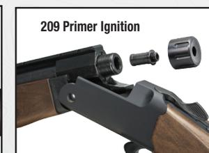
**ADAPT™ BREECH SYSTEM** - The primer adapter eliminates the need for threading inside the barrel which is the leading cause of seized breech plugs. The Adapt™ Breech System also allows you the ability to change out your primer adapter to different configurations, which will optimize ignition performance with your propellant of choice.
