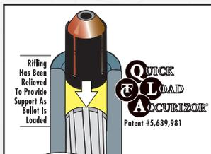
**QUICK LOAD ACCURIZOR®** Muzzle System QLA® allows the shooter to quickly and easily load his/her muzzleloader by incorporating a false muzzle design into the end of the barrel.
