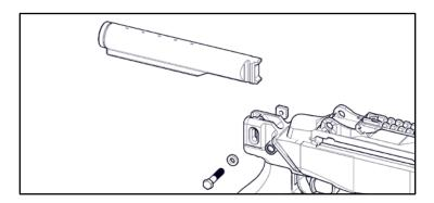
**Stock Info** - The stock and receiver extension are both of the "MilSpec" diameter. As such, the stock may be used on any other MilSpec sized extension, and any other MilSpec stock may be used on M1A Modstock.
