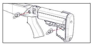
Compartment Storage - The trapdoor compartment (water-resistant) is designed to hold a pair of AA batteries, while the cheekweld compartments (waterproof) are designed to hold four CR123 "Surefire" batteries on each side, but are capable of holding AA batteries, ear plugs, bore snakes, lube, etc.
