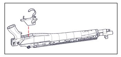
Slide Receiver Extension Tube into Adapter dovetail. Adjust to preferred height and secure using Square Nut, M14 Special Bolt, and Washer.
