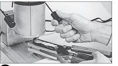
**6** Fill the mold through the sprue plate, puddle enough so all of the sprues are connected. Leave a ¼" to ½" gap between the sprue plate and the nozzle when filling the mold cavities. **NOTE** Resting the mold on the sprue plate while filling will pressure cast the cavities and may push molten material into the vent grooves, causing flashing on bullet.
