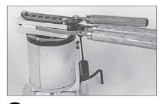
Pre-heat your mold by laying it on top of your lead melter or dip the corner of mold into molten metal for at least 30 seconds. If the lead sticks and solidifies on the mold block it's not hot enough.
