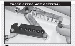
Lubricate your mold using beeswax or Permatex® anti-sieze lubicant or equivalent. DO NOT USE Lee Liquid Alox as it will bake on the mold surface, preventing proper closure. Do not use paraffin wax as it does not provide adequate high temperature lube and tends to migrate to the cavities, causing wrinkled bullets.
