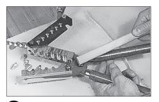
Open the mold and drop the bullet onto a soft cloth. (An old towel works well.) It may require a few taps on the handle bolt to free the bullets.
