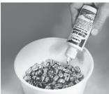
Alox. This places the lube where needed, on the surfaces that rub against the bore. Lead bullets must be lubricated or your gun will be fouled with lead and accuracy will be poor.
