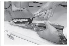
Immediately after sprue solidification operate the sprue lever if equipped or rap the sprue tang with a wood dowel. (A frosted surface will appear on the sprue puddle upon solidification).
