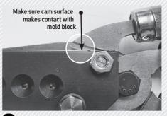
5 If you are using a six cavity mold be certain the sprue lever cam surface is in contact with the mold block side and there is a gap between the edge of the sprue plate and the formed stop on the sprue lever.
