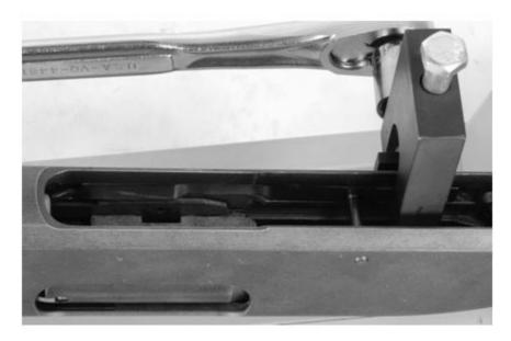
The staking tool in the proper position.
