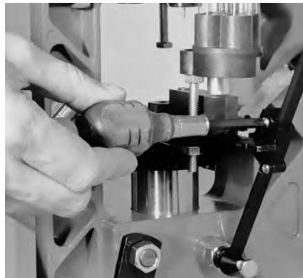
**Tighten top screw. Adjust shell insertion pressure with bottom screw.**
