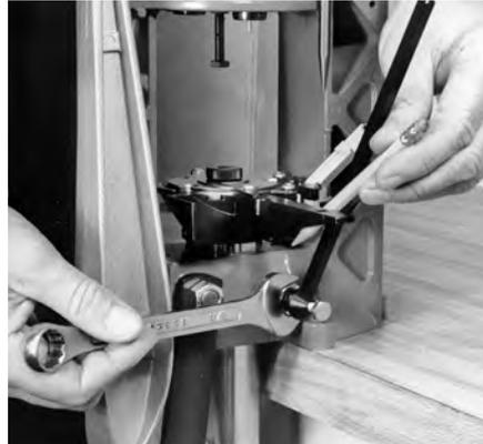
upper most ram travel, place a case in front of the shell slider, cycle lever, again place case in front of slider, cycle lever. If the case collides with the case in shell plate, remove feed rod and unscrew feed bracket one or more full turns. When tightening feed bracket, **be sure to allow  $\frac{5}{16}$ " clearance between carrier tongue and square rod—about the thickness of a pencil.**
