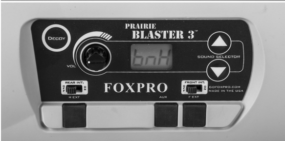
Battery Chemistry NiMH Cells Setting
