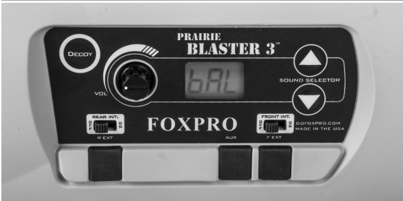
Battery Chemistry Alkaline Cells Setting
