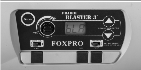
Battery Chemistry Lead Acid Battery Setting
