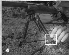
To adjust each leg, loosen the compression collar and adjust legs the desired height, then retighten. (See picture 4)
