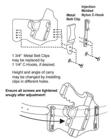
A belt up to 1  $\frac{1}{4}$ " is quickly and easily threaded through the optional C-Hooks.
