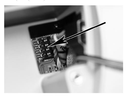
The image shown above is looking directly down onto the switch in the battery compartment. The available positions (ON/OFF) are noted. The ON position is selected by moving the switch to the right. The OFF position is selected by moving the switch to the left. Each of the four switches are marked 1-4. When referring to the matrix below, be sure that you modify the switches starting with 1 and then continue through number 4.
