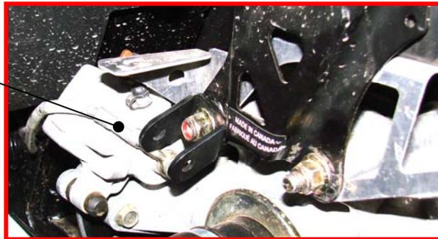
Align the Kolpin Top Bracket and the Kolpin Bottom Bracket using the Lock Out Rod
