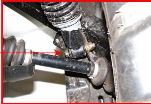
3. Put the OEM bolt you just removed through the Kolpin Bottom Metal Bracket (smaller of the two brackets) provided in the kit, and place the bolt back through the shock. Do not fully tighten yet as you will have to swivel the bracket to meet up with the Top Bracket.
