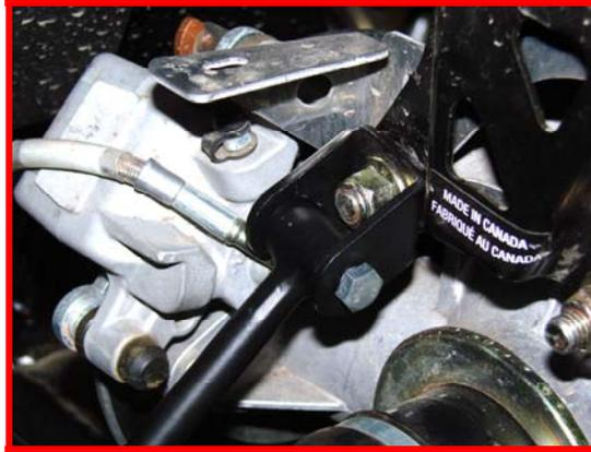
8. Now, swivel the Lock Out Rod to meet the Bottom Bracket on the shock. Using the pin lock provided, pin the Lock Out Rod to the Bottom Bracket. Tighten the Bottom Bracket Securely after pinning.
