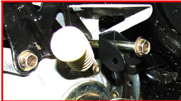
Make sure the nut is above this brake line, located on the left rear side of the machine.
