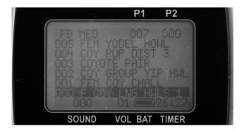
The TX9 will display 000 for both P1 and P2 when you first turn it on. In order to use the preset buttons, you must first assign a sound and volume to each.
