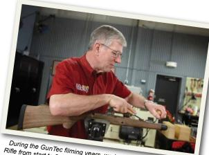
During the GunTec filming years, we build a Nearly-Perfect Safari Rifle from start to finish -- truing up the action through finishing and checkering the stock.
