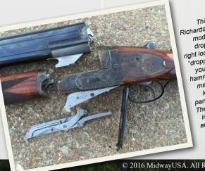
This Westley Richards "Ovundu" model features droplocks. The right lock has been "dropped out" and you can see the hammer, sear and mainspring. The left lock is only partially removed. The only parts left inside the action are the firing pins and the trigger.
