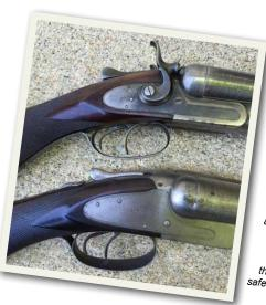
These two early L.C. Smith shotguns, made in the 1880's, are good examples of the hammer-type and hammerless sidelocks. Note that the hammer and the firing pin are inside the action on the lower gun, and there is a sliding safety on the tang.
