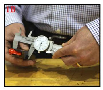
Small frame (Pre 2005) Witness magazines, as pictured above measure approximately 0.796" thick (fig. 1A) and approximately 1.25" long (fig. 1B).
