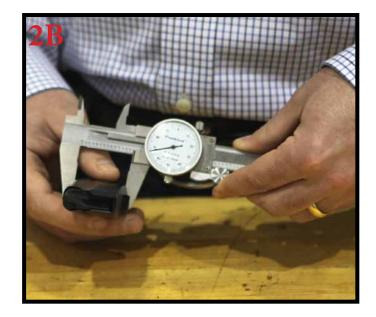
Large frame (Post 2005) Witness magazines, as pictured above measure approximately 0.843" thick (fig. 2A) and approximately 1.369" long (fig. 2B)
