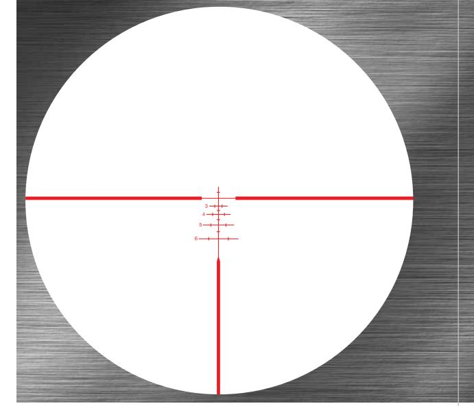
Reticle design parameters: Sight-in distance/Zero: 200 yards (main horizontal bar) Altitude: 2000 feet Pressure @ Altitude: 27.48 (in Hg) Humidity: 78% Temperature: 59 deg F Sight height above bore: 1.8 inches Incline angle: 0 Spin drift: 0 Applications: General hunting Mid-range shooting
