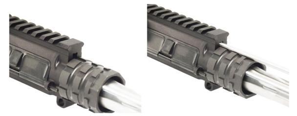
If the groove aligns and the gas tube can be inserted into the upper receiver, install gas system according to manufacturer's instructions, and proceed to step 6.
