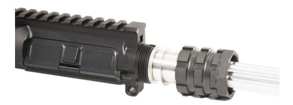
4. Tighten barrel nut and inspect alignment of barrel nut groove and gas tube port in upper receiver (see below)
