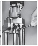
Push the assembly onto the ram's end. Tighten the clamp screw with a hex wrench.
