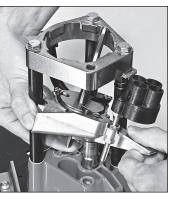
Push the action rod up through the top of the press and continue rotation to level position. Be sure to keep the primer trough pin behind the right rear column.
