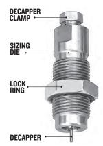
Screw the full length sizer in until it touches the shell plate, and tighten the lock ring finger tight. The decapper is retained by a collet. Should it be overstressed by an obstruction; it simply slides up without damage. To reset, loosen the decapper clamp and position the decapper flush with clamp end and retighten. **Considerable torque** may be necessary. A  $\frac{1}{2}$  and  $\frac{3}{4}$  wrench are needed.
