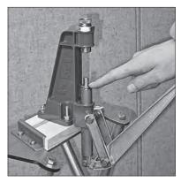
(a) Install push pin into shell holder slot.
